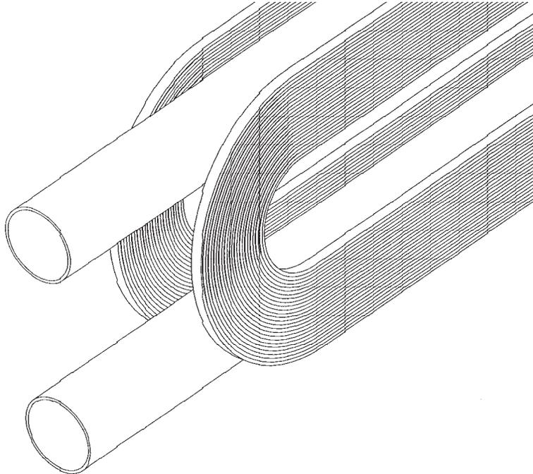
FIG. 1. Arrangement of two racetrack coils to produce dipole fields in two apertures.
