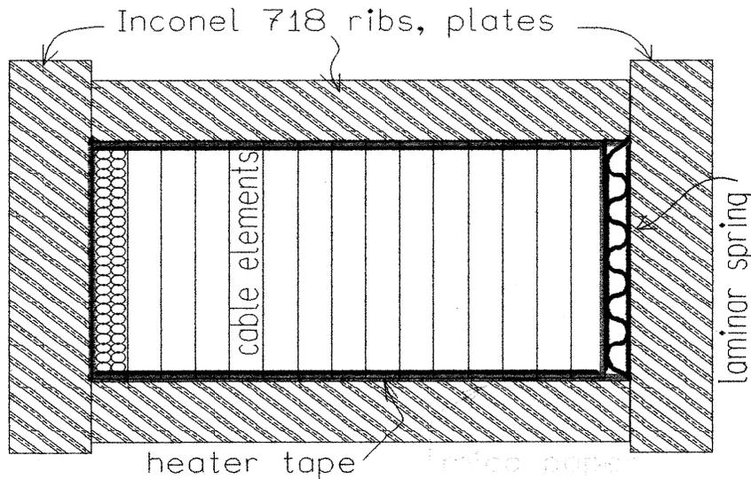
FIG. 8. Cross section of one conductor block and Inconel support structure.
