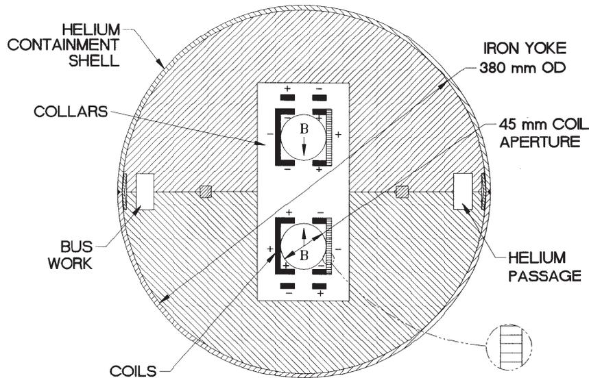
FIG. 2. Cross section of common coil magnet including racetrack coils, yoke, and correction coils.
