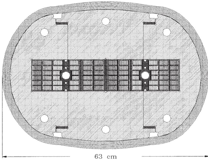
FIG. 7. Cross section of high-field dual bore block dipole.
