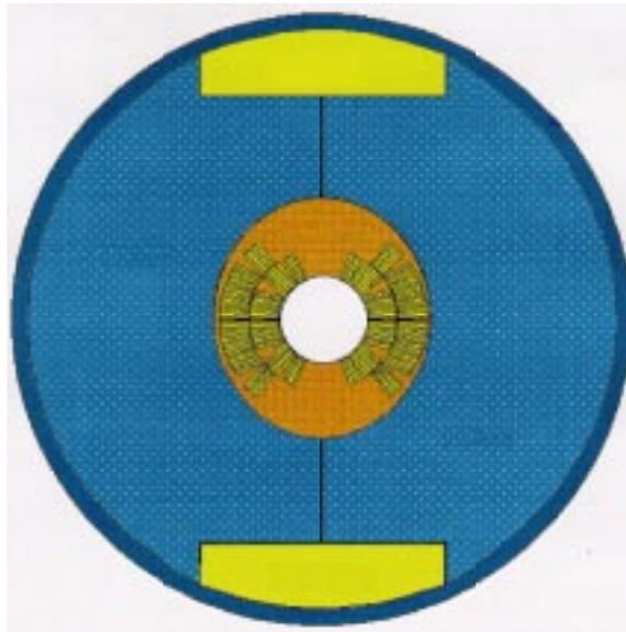
FIG. 6. Initial design cross section for a high-field Nb3Sn cos-theta dipole.
