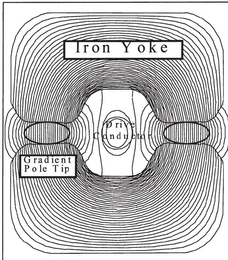
FIG. 4. Yoke and conductor for transmission line magnet, showing lines of flux.
