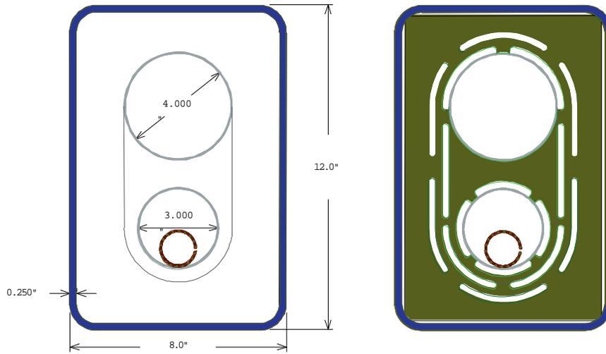
FIG. 5. Cross-sections of the helium supply and return and current return for the transmission line magnet.
