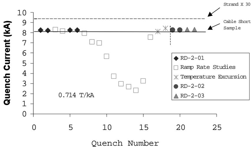
FIG. 3. Quench performance of 1 m LBL common coil magnet.
