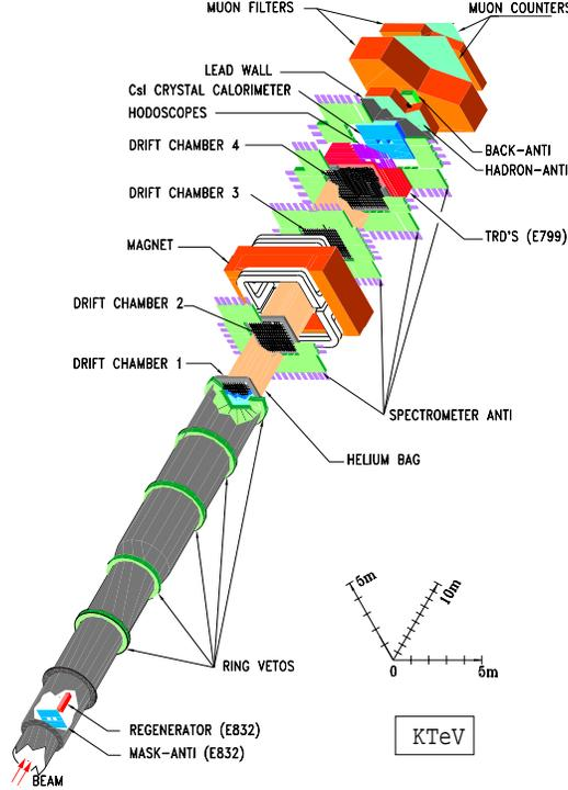
FIG. 2. 3D View of the KTeV Detector.
